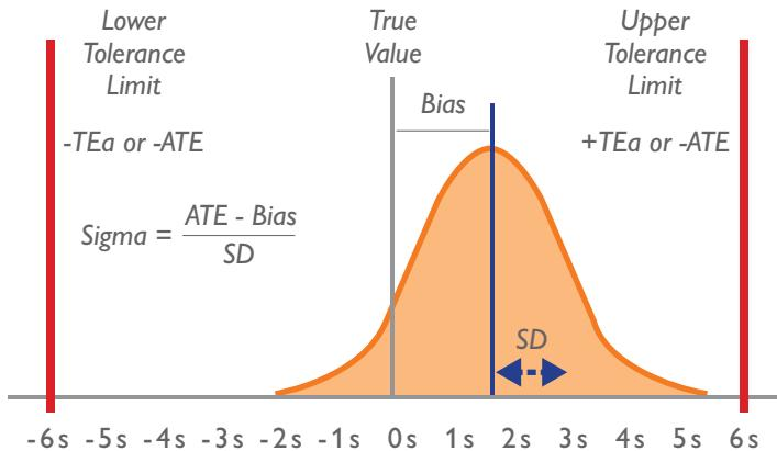
**Figure 1.** Predicting defects using imprecision (CV), inaccuracy (Bias) and total allowable error (TEa)
